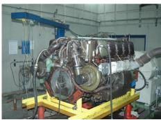
Diesel Engine Test Bench
