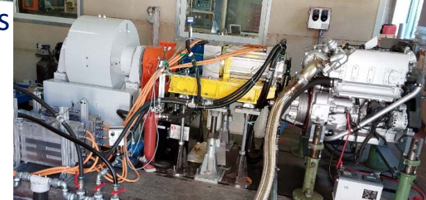
Fig.3: Experimental setup FNM 300HPE + 2 PARKER GVI at STEAMS Test bench
